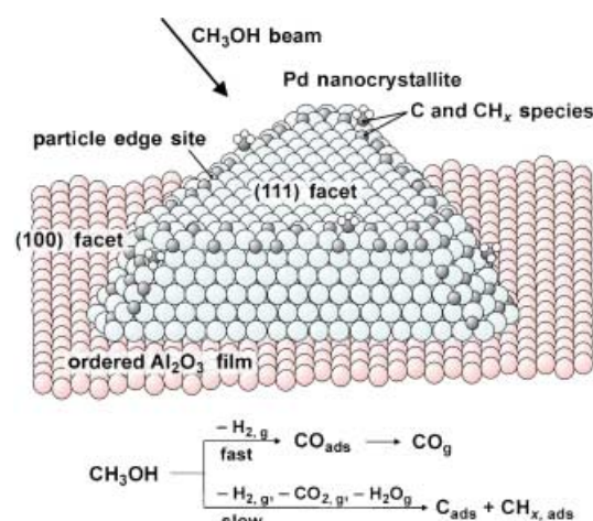
Figure 1. Schematic representation of the supported Pd nanoparticles and the blocking of defect sites by carbon species during methanol decomposition.
